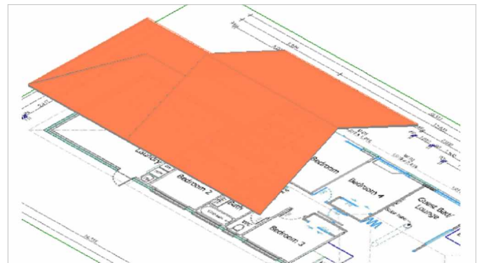
Remove Roof Cladding x 135m2
